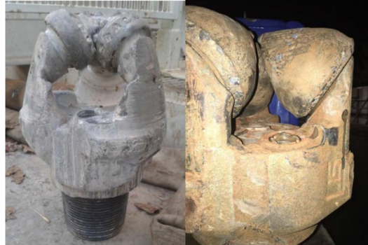
Figure 8. Roller cone bits completely destroyed after drilling the St1 well (Cardoe et al. 2021).
