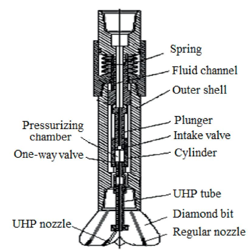
Intensifier that generates high pressure water jet in the downhole conditions.
