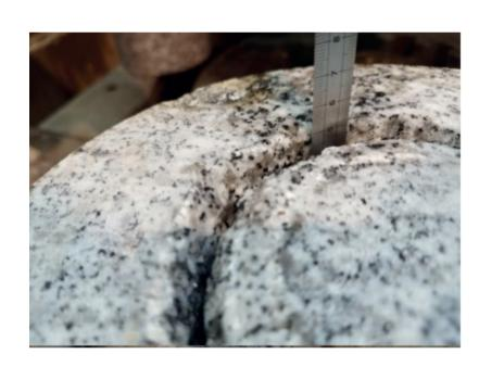
(L) Demonstration of increased drilling rate with HPWJ; (R) A peripheral groove slotted in Sidobre (UCS 150 MPa).
