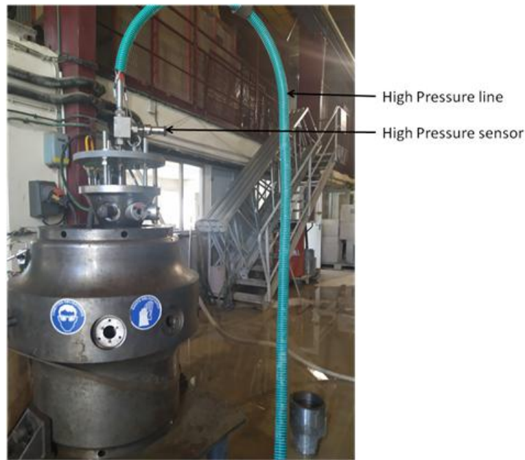
Figure 4: The high pressure impact cell modified to accommodate the high pressure water jetting experiments.
