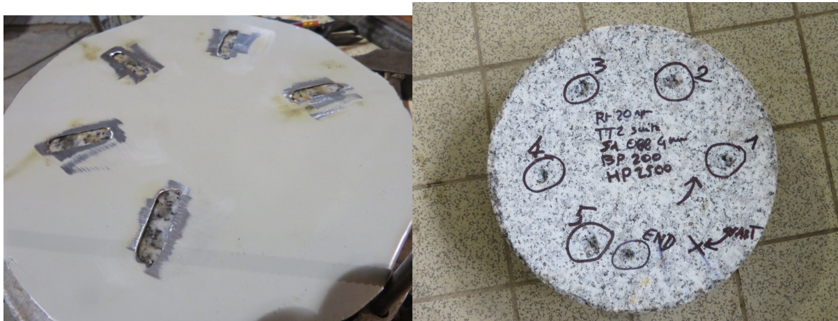
Figure 12: The steel plate fabricated to isolate the impact zone to 1 cm width and the resulting craters created localized around the 1 cm slots
