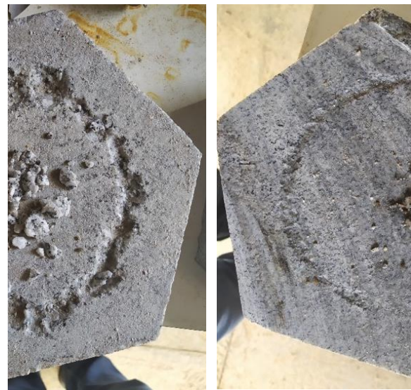
Figure 23: Different susceptibilities of two granite specimens of ~200 mm across (Left: Sidobre, Right: Kuru Grey) to HPWJ grooving as rock specimen rotates under the jet with 180 MPa of HPWJ chamber pressure, 10 MPa back pressure, 4 mm stand-off distance and 4 RPM rotation speed. The nozzle is Karcher forme 1 of 1.0 mm orifice.
