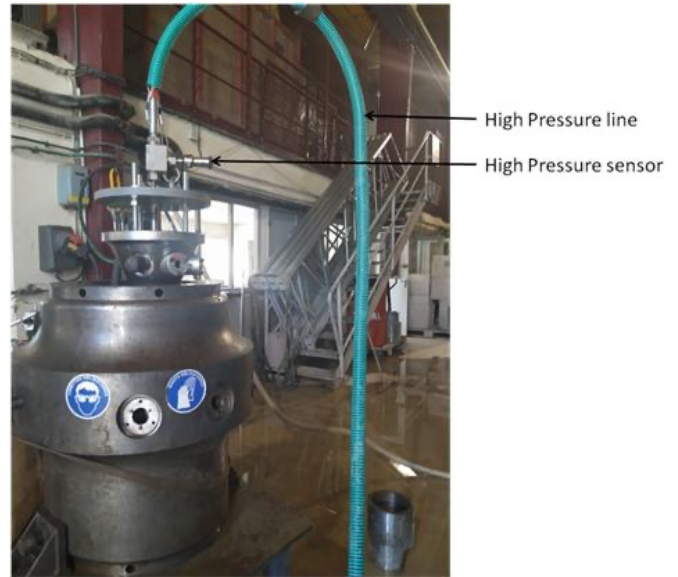
Fig. 4: The high-pressure impact cell modified to accommodate the HPWJ experiments. The high-pressure transmission line is connect to a pump that can generate a maximum pressure of 250 MPa.
